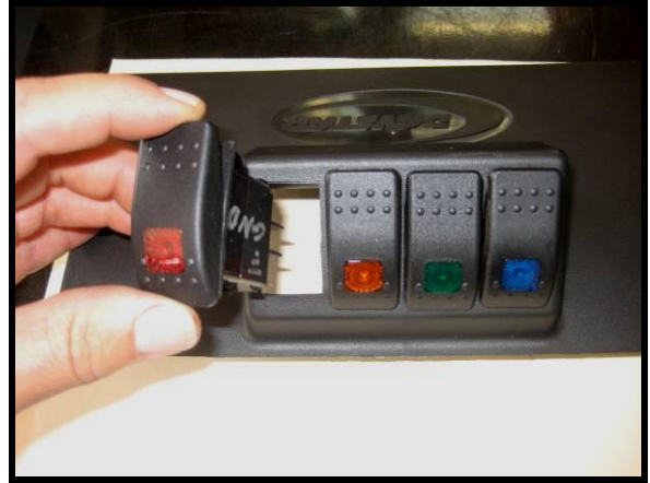
Insert switches from front side and wire as needed.
