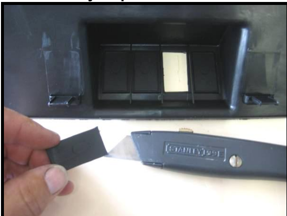
Carefully cut panel from back side with razor knife for desired switches.
